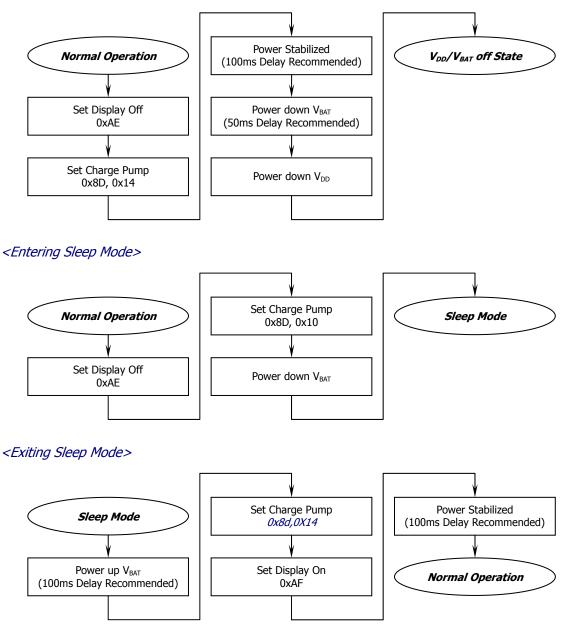
Internal setting (Charge pump) void sh1106()
